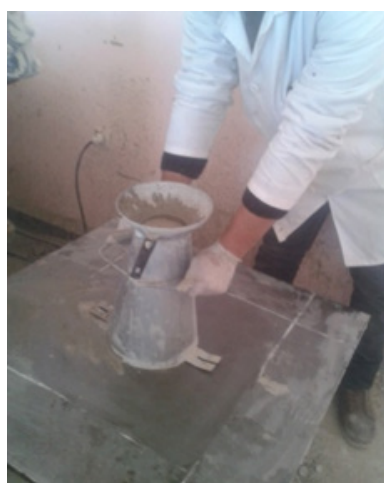
Fig. 5 Self-compacting concrete sprawl test
