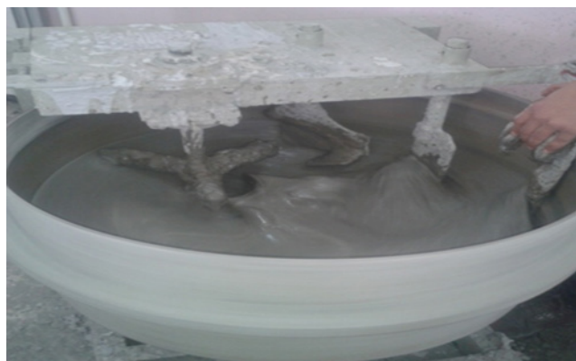
Fig. 3 Concrete mixing in the self-compacting concrete
