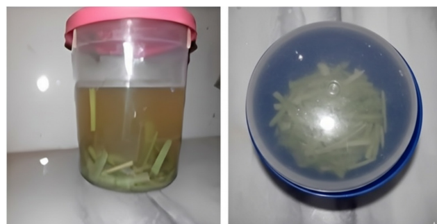
Fig. 2 Preparation and soaking of natural fibers extracted from date palm residues for use in earth block reinforcement
