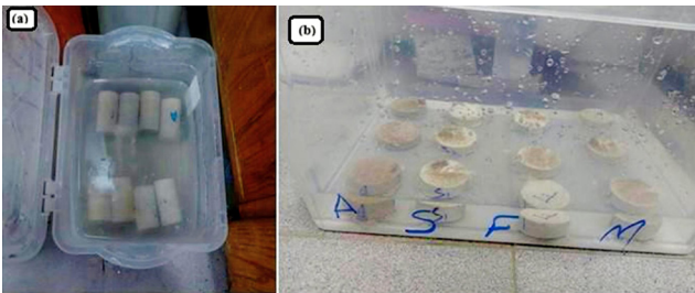
Fig. 8 Sample preparation for aging tests: (a) indicate the immersion of samples in saline solution in preparation for testing after aging; (b) show the prepared samples for testing
