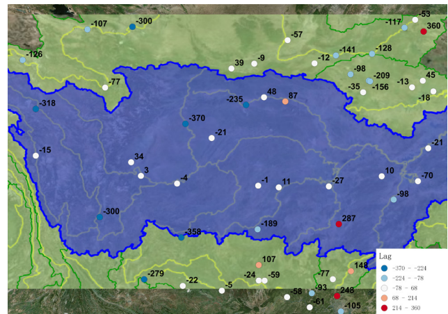
Fig. 13 Phase lags of reliable stations in the Yangtze River basin
