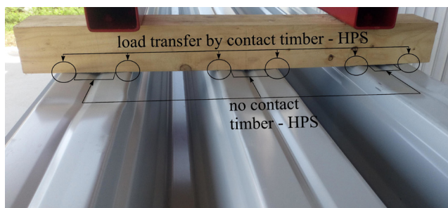
Fig. 9 Load transfer from timber beams on HPS
