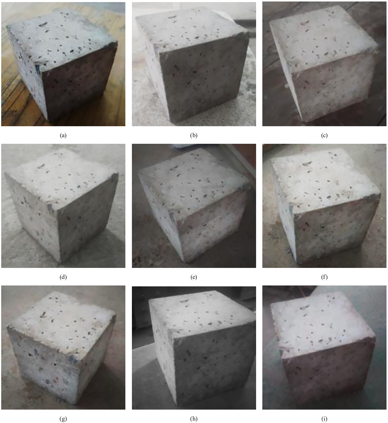
Fig. 8 Surface observation of the microwave-cured specimen (MC1000-30) during the sulfate resistance test for 9 cycles: (a) Cycle #1, (b) Cycle #2, (c) Cycle #3, (d) Cycle #4, (e) Cycle #5, (f) Cycle #6, (g) Cycle #7, (h) Cycle #8, (i) Cycle #9
