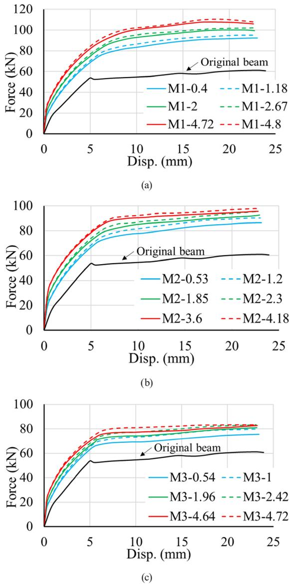
Fig. 16 The force-displacement results of strengthened beams
