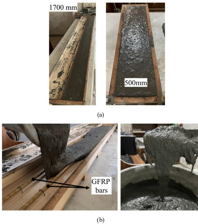
Fig. 3 (a) The mold of 500 and 1700 mm samples (b) Mortar of specimens
