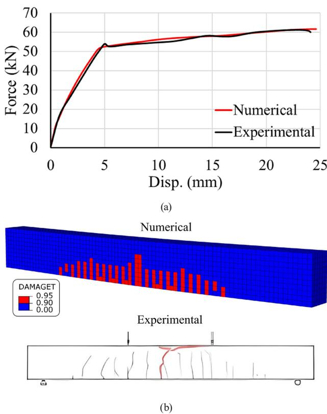
Fig. 11 Comparison of numerical and experimental results
