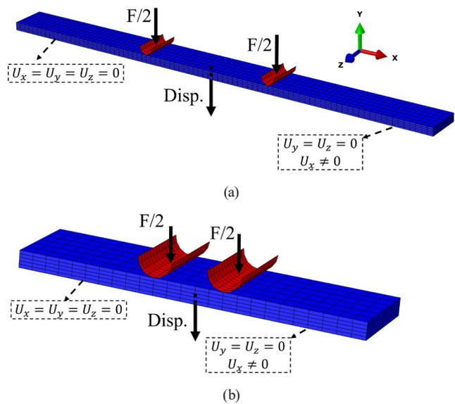
Fig. 12 Boundary conditions of the meshed models for the length of
