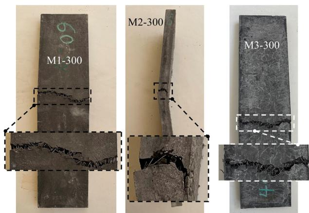
Fig. 7 The failure of models without GFRP
