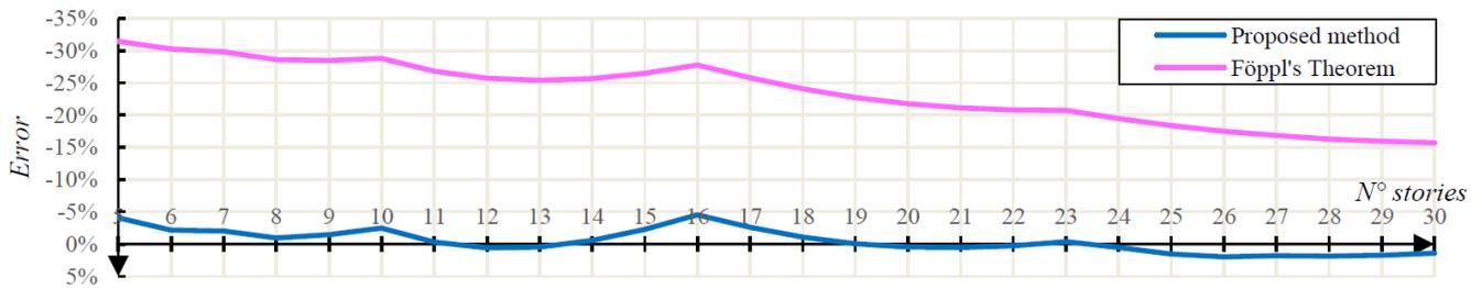
Fig. 5 Accuracy in the calculation of the critical global buckling load using the proposed method and Föppl's theorem
