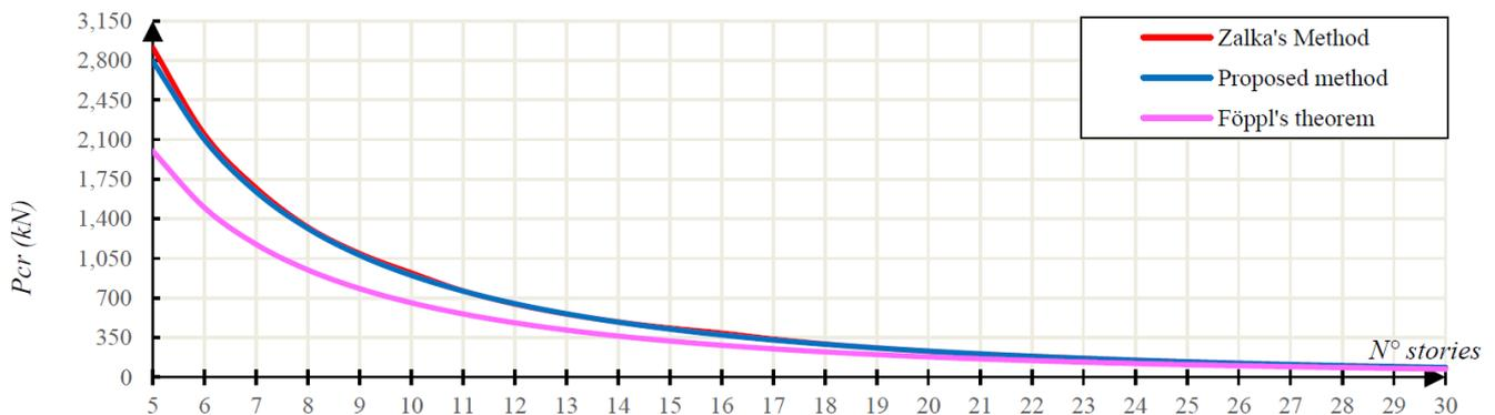
**Fig. 4** Critical global buckling loads obtained using Zalka's method [48], Föppl's theorem, and the proposed method
