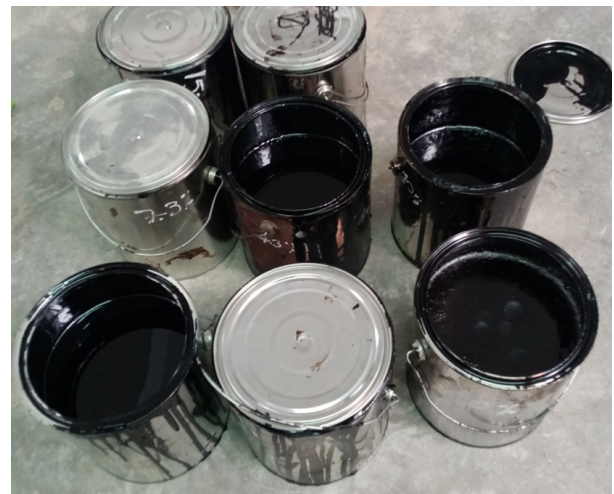
Fig. 2 Disposal of TPU-modified asphalt cement
