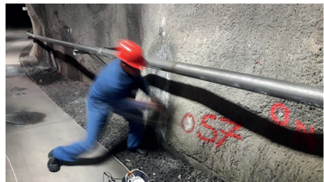
Fig. 3 Seismic wave propagation using a hammer at the source point on the tunnel wall
