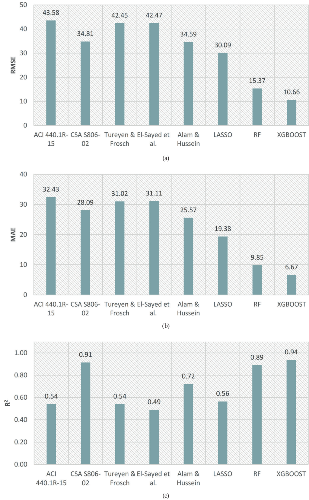
Fig. 8 Results comparison between all test samples for shear strength prediction of FRP-reinforced concrete beams: (a) RMSE; (b) MAE; (c) R 2
