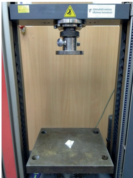
Fig. 3 ZWICK Z020 tensile tester before the test
