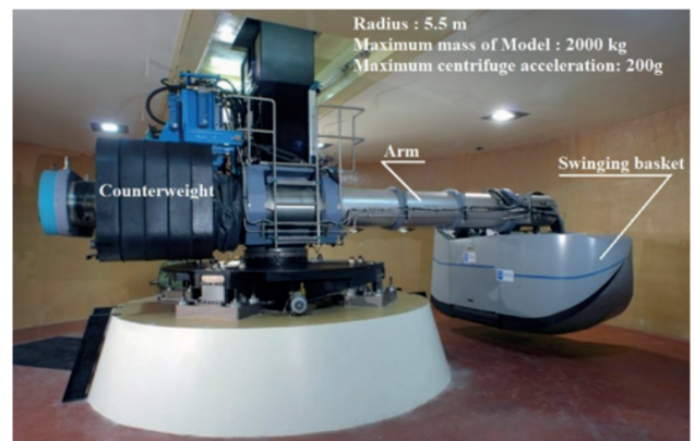
Fig. 2 Geotechnical centrifuge of the IFSTTAR
