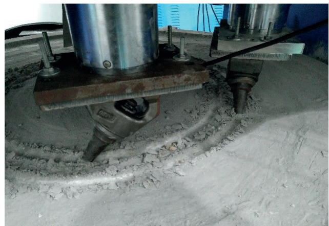
Fig. 17 Coal-rock cutting simultaneously by two conical picks
