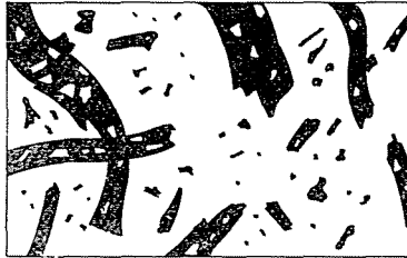
Fig. 2. Scheme of complex soap structure in lubricating greases
