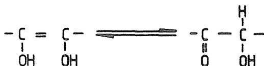
Fig. 2. Enediol class keto-enol tautomerism in Vitamin-C
