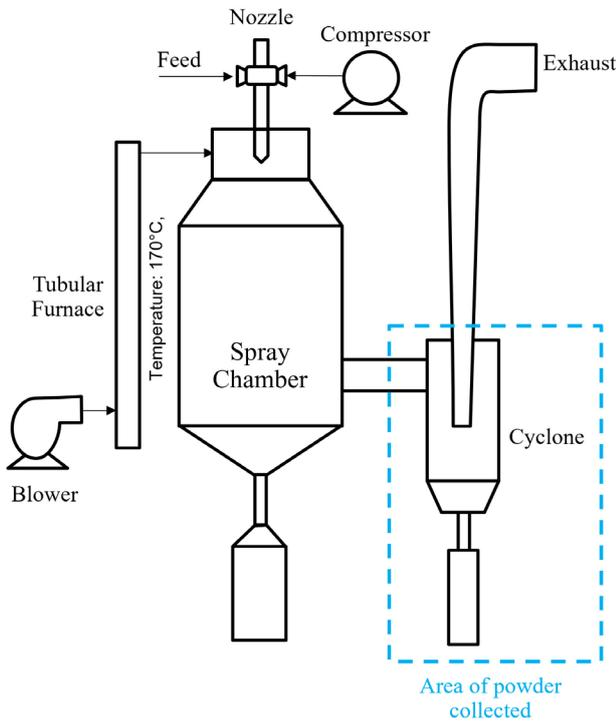
Fig. 1 Spray drying system
