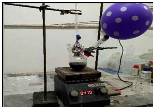
Fig. 1 Experimental setup for preparation of alumina-nZVI composite in laboratory
